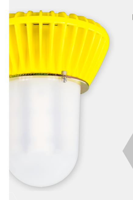
Explosion-proof LED luminaire of an ELHB Ex type is characterised by high luminous flux. It is a compact light source with ultra-bright LEDs installed for high intensity of lighting and with a wide angle of light distribution. Diodes are enclosed in a corrosion-resistant housing made of high-quality aluminium and a lampshade made of suitable plastic. LEDs do not emit UV light or heat.
